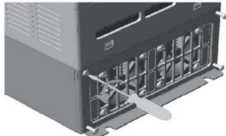
旋松端盖板螺钉
